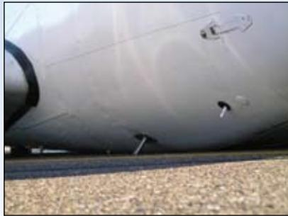
*Once the sparks stop flying and the airplane grinds to a sickening halt, damage—major and minor—can be found everywhere. The flaps, lower left, are usually trash and bits and pieces of belly-mounted antennas will be found smeared along the runway.*
